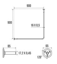
Tube Ø 16 x 0,5 mm. Can be cut to size. 2 long sliding wall flanges.
