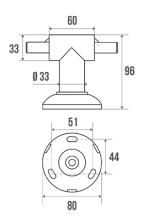
White polyamide (nylon). Tube Ø 33 mm. White flange border. Concealed fixings.
