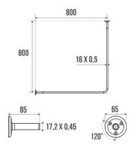
Tube Ø 16 x 0,5 mm. Can be cut to size. 2 long sliding wall flanges.
