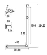
Composite material: White synthetic resin + aluminium profile. Tube Ø 33 mm. With shower rail slider bracket. White flange border and central body. Concealed fixings. Delivered unassembled. Allows either right or left-handed configuration.
