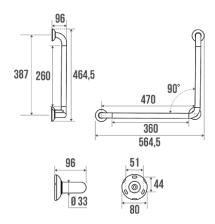
Composite material: White synthetic resin + aluminium profile. Tube Ø 33 mm. White flange border and central body. Concealed fixings.
