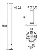
Tube Ø 16 x 0,5 mm. Can be cut to size. 2 long sliding wall flanges.
