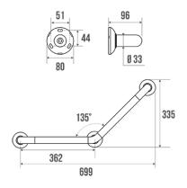
Composite material: White synthetic resin + aluminium profile. Tube Ø 33 mm. White flange border and central body. Concealed fixings.
