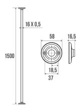
Tube Ø 16 x 0,5 mm. Can be cut to size. 2 sliding wall flanges.
