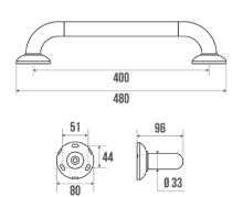
Composite material: White synthetic resin + aluminium profile. Tube Ø 33 mm. White flange border and central body. Concealed fixings.
