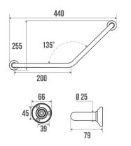
Symmetrical. Concealed fixings. Chrome and nickel-plated brass tube Ø 25 mm. Bright chrome-plated resin flanges and cover plates.
