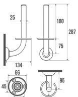
Concealed fixings. Steel wire  $\varnothing$  6 mm. Synthetic resin flange and cover plate. Blue (RAL 5002) cover plate. Steel tube  $\varnothing$  25 mm.
