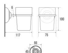
Wall-mounted. Concealed fixings. Frosted translucent resin glass. Steel wire Ø 6 mm. Synthetic resin flange and cover plate. Red (RAL 3003) cover plate. Steel tube Ø 25 mm.
