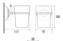
Wall-mounted. Concealed fixings. Frosted translucent resin glass. Steel wire Ø 6 mm. White synthetic resin flange and cover plate. Steel tube Ø 25 mm.
