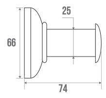
Concealed fixings. Synthetic resin flange and cover plate. Red (RAL 3003) cover plate. Steel tube  $\varnothing$  25 mm.
