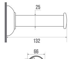
Concealed fixings. White synthetic resin flange and cover plate. Steel tube  $\emptyset$  25 mm.
