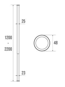
White epoxy-coated aluminium tube  $\varnothing$  25 mm with suction cups. Cannot be shortened.
