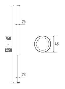
White epoxy-coated aluminium tube Ø 25 mm with suction cups. Cannot be shortened.
