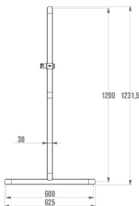
Multi-component : Nylon + steel profile. Elliptical tube 38 x 25 mm for a better grip.
