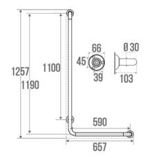
Supplied with universal clip-on shower rail slider bracket in white ABS. White epoxy-coated aluminium tube. White resin cover plates. 90° right corner.
