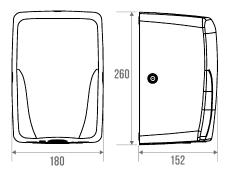
Rated voltage: 220 V-240 V. Rated power: 500 to 1150 W. Outlet airspeed: 215 to 380 km/h.
