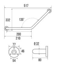
3 fixing points. 200 x 200 mm symmetric grab bar. Bright polished 304 stainless steel tube  $\emptyset$  32 mm. Bright polished stainless steel cover plates and flanges. Wall fixings included. Incompatible in chlorinated environment.
