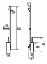
Elliptical aluminium tube 38 x25 mm, polymer fixing covers. Concealed fixings.
