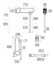
Elliptical tube 38 x 25 mm in anthracite grey epoxy-coated aluminium.
