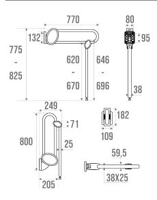
Elliptical tube 38 x 25 mm in white epoxy-coated aluminium. Wall flange, cover plate, joint in white synthetic resin and mat chrome-plated side plates. With integrated support prop, adjustable height.
