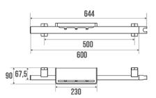
Elliptical aluminium tube 38 x25 mm, polymer fixing covers. Concealed fixings.
