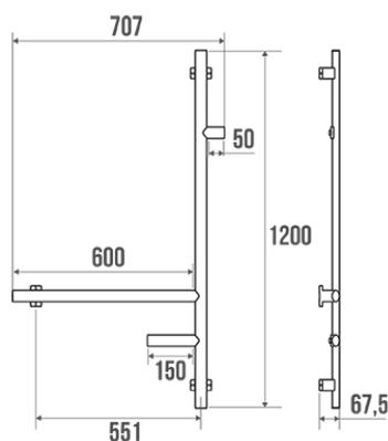
Elliptical aluminium tube 38 x25 mm, polymer fixing covers.
