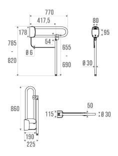
White epoxy-coated aluminium tube Ø 30 mm. Synthetic resin flange. With integrated support prop, adjustable height with a system of jack. Concealed fixings. Corrosion-resistant warranty.
