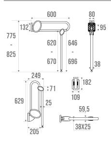
Elliptical tube 38 x 25 mm in white epoxy-coated aluminium. Wall flange, cover plate, joint and side plates in white chrome-plated synthetic resin.
