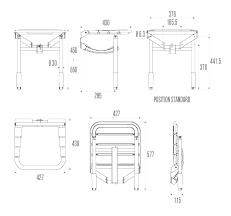
Foldaway seats with legs whose height can be adjusted to 100 mm and that are equipped with smooth shoes for 450, 500 to 550 mm height (it adjusts to the gradient of the shower base)
