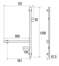
Elliptical aluminium tube 38 x25 mm, polymer fixing covers.
