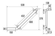
Elliptical aluminium tube 38 x25 mm, polymer fixing covers. Concealed fixings.
