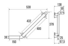
Elliptical aluminium tube 38 x25 mm, polymer fixing covers.
