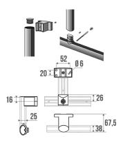
Multi-components: Polymer link pieces. For assembly with Arsis straight sections. Adapted to customized layouts.
