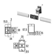
Multi-components: Polymer link pieces. For assembly with Arsis straight sections. Adapted to customized layouts.
