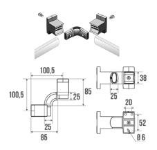
Multi-components : Polymer link pieces. For assembly with Arsis straight sections. Adapted to customized layouts.
