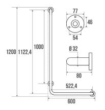
Bright polished 304 stainless steel tube Ø 32 mm. Bright polished stainless steel cover plates and flanges. 3 fixing points. Angle to the left. ABS slider bracket for shower handset. Concealed fixings. Wall fixings included. Incompatible in chlorinated environment.
