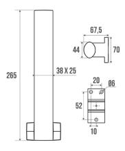
Elliptical anthracite grey aluminium tube  $38 \times 25 \text{ mm}$ . Anthracite grey synthetic resin cover plates.
