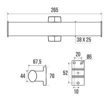
Elliptical anthracite grey aluminium tube  $38 \times 25 \text{ mm}$ . Anthracite grey synthetic resin cover plates.
