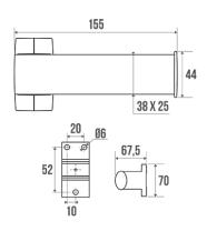
Elliptical anthracite grey aluminium tube 38 x 25 mm. Anthracite grey synthetic resin cover plates.
