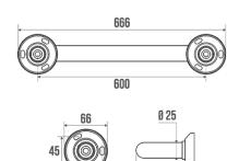
Chrome and nickel-plated brass tube Ø 25 mm. Fixings and cover plates in bright chrome-plated synthetic resin.
