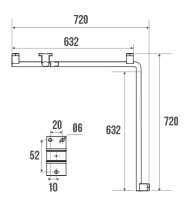
Elliptical tube in anthracite grey epoxy-coated aluminium, 38 x 25 mm.
