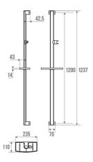
Elliptical tube in bright anodized aluminium, 38 x 25 mm. Chrome-plated synthetic resin cover plates.
