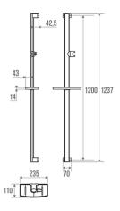
Elliptical tube in white epoxy-coated aluminium,  $38 \times 25 \text{ mm}$ . Mat chrome-plated synthetic resin cover plates.
