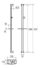
Elliptical tube in white epoxy-coated aluminium,  $38 \times 25$  mm. White synthetic resin cover plates.
