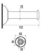
Concealed fixings. Synthetic resin wall fixings and cover plates. Blue cover plates(RAL 5002). Steel tube Ø 25 mm.
