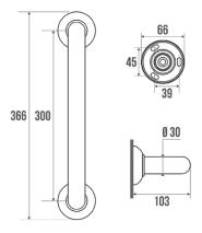
White aluminium tube Ø 30 mm, synthetic resin wall fixings and blue synthetic resin cover plates (RAL 5002), Ø 66 mm.
