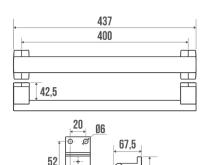
Elliptical tube in anthracite grey epoxy-coated aluminium, 38 x 25 mm with graffiti effect finish. Anthracite grey synthetic resin cover plates.
