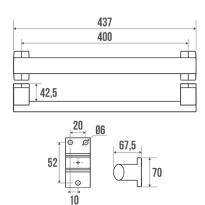
Elliptical tube in anthracite grey epoxy-coated aluminium, 38 x 25 mm with wooden effect finish.
