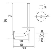
Chrome and nickel-plated brass tube. Polyamide flanges and chrome-plated brass cover plates. Concealed fixings.
