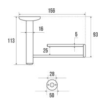
Chrome and nickel-plated brass tube. Polyamide flanges and chrome-plated brass cover plates. Concealed fixings.
